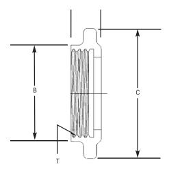
Material - Cast High Standard Magnesium Bronze per ASTM B584
