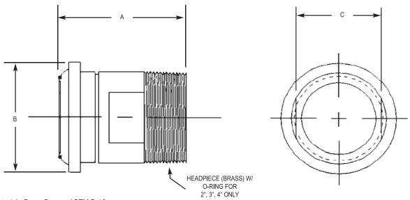
Material - Brass Bar per ASTM B-16
