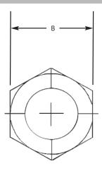
Material - Brass Bar per ASTM B16
