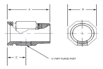
Material - Brass Bar per ASTM B16
